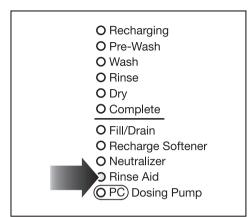
Rinse aid does not need to be refilled until the "Rinse aid" indicator light comes on in the display.
